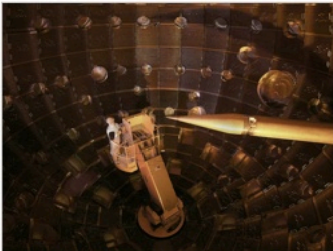
The interior of the National Ignition Facility's target chamber, where researchers plan to use 192 giant lasers to ignite a pinpoint fusion reaction. Credit: LLNL/DOE
